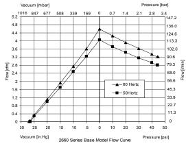
uum [in.Hg] 2660 Series Base Model Flow Curve
